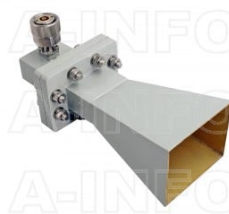
LB-137-10-C-7 Standard Gain Horn Antenna 5.85-8.2GHz 10dB Gain 7mm
