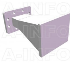
LB-137-10-ASPO Standard Gain Horn Antenna 5.85-8.2GHz 10dB Gain Rectangular Waveguide Interface
