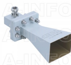
LB-137-10-C-NF Standard Gain Horn Antenna 5.85-8.2GHz 10dB Gain N Type Female
